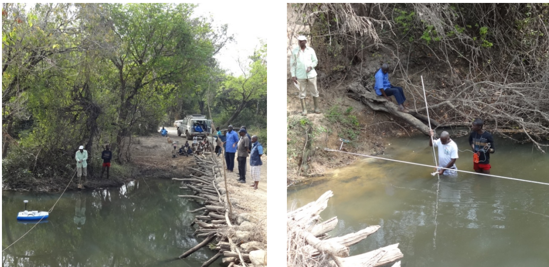
Fig. 8 Discharge measurement Irradougou gauging station with ADCP and moulinet
