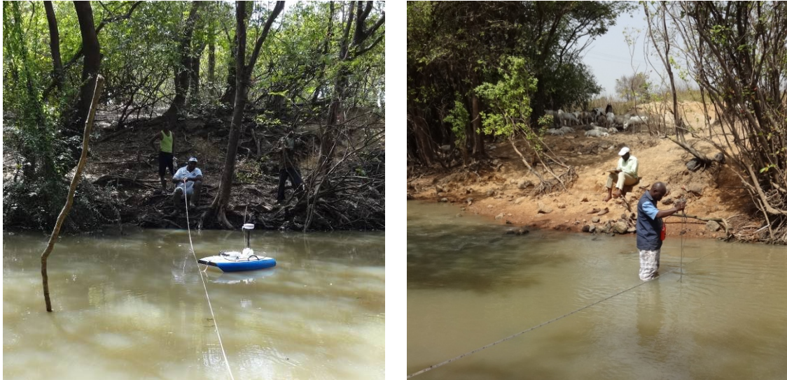
Fig. 5 Discharge measurement at Samatiguila with ADCP and moulinet
