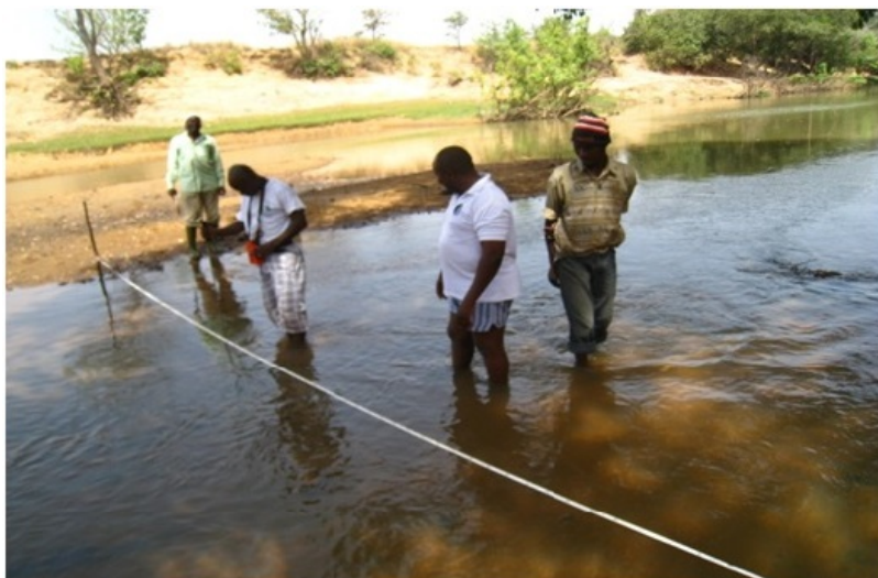
Fig. 3 Discharge measurement at Kouto River with moulinet (classic current meter)
