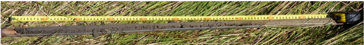
Figure 5: Groundwater affected soil with gleyic properties from the area northwest of Lusaka International Airport
