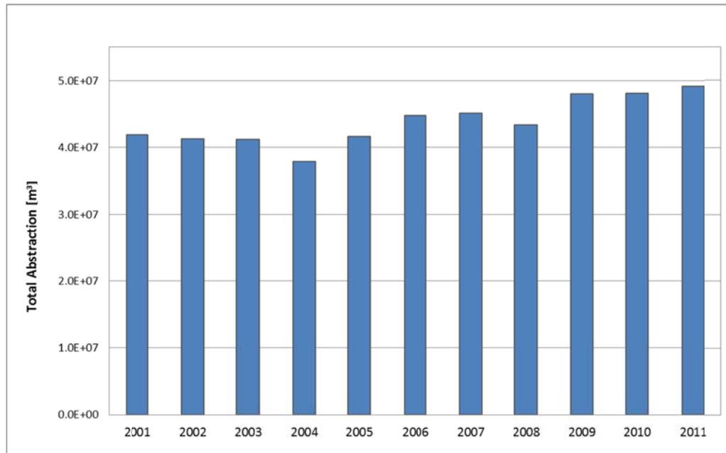
Figure 14 Groundwater abstraction per year from the LWSC boreholes for the last ten years from 2001 to 2011 (Data Source: Lusaka Water and Sewerage Company)
