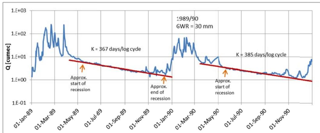
Figure 20 Example of determination of recharge at station 5-025 Chongwe using Meyboom's method
