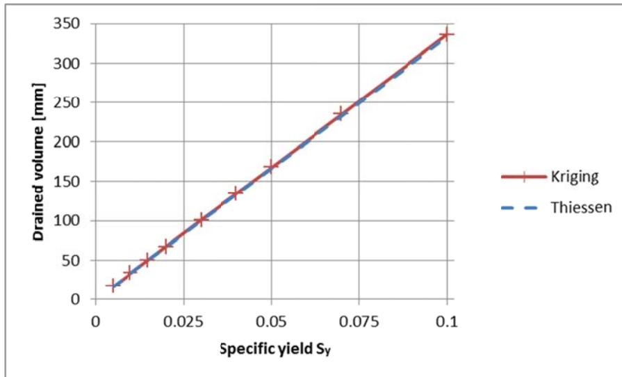
Figure 23 Estimated volume of drained pore space during the 2009 dry season (April to October) for the Lusaka Dolomite Plateau as a function of specific yield  $S_y$ ; The two different lines show results based on interpolation of point data using Kriging and Thiessen polygon methods.
