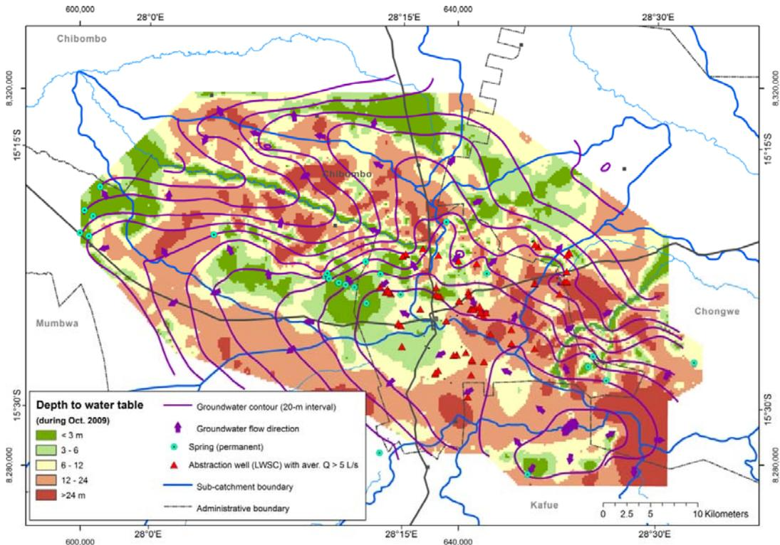
Figure 18 Depth to water table and groundwater flow in the Lusaka Plateau area during October 2009
