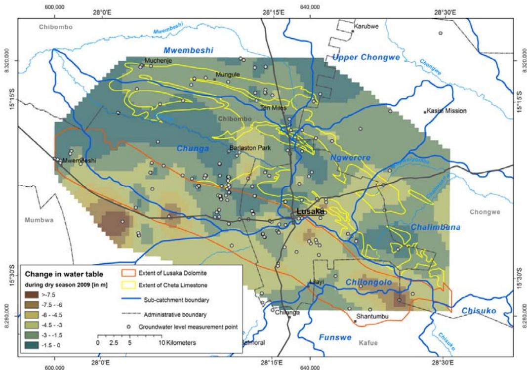
Figure 22 Drop in groundwater tables between April 2009 and October 2009 (based on Kriging interpolation method of point observations)
