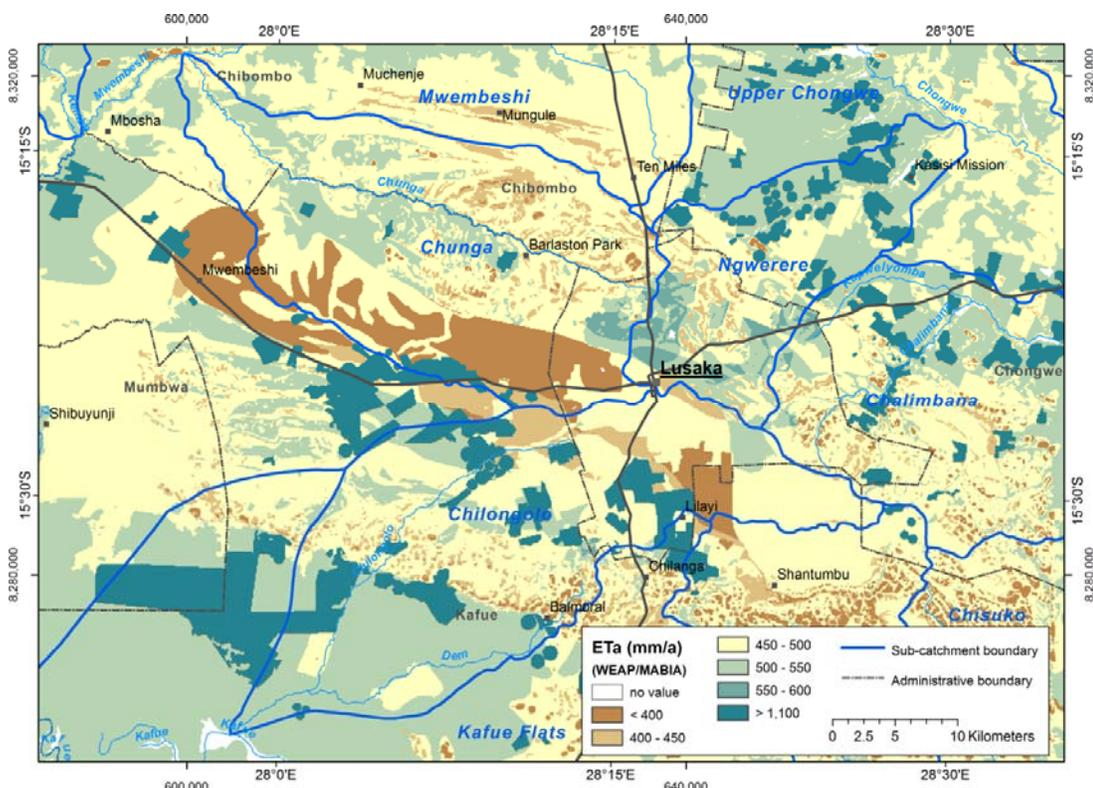
Figure 4 Actual Evapotranspiration  $ET_a$  in mm/a for the Lusaka region in the reference year 1989/90 calculated with the WEAP/MABIA-model using meteorological data from Lusaka International Airport. Areas with  $ET_a > 1100$  mm represent commercial agricultural land under dry season irrigation (after Hennings 2012).
