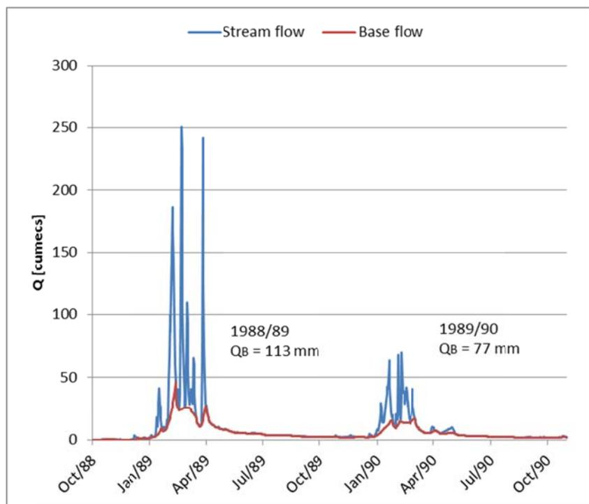
Figure 19 Example of base flow separation with PART (station 5025-Chongwe for hydrological years 1988/89 and 1989/90)
