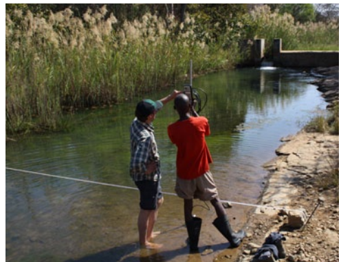
Stream flow calibration measurement at Kapiriombwa Stream east of Lusaka
