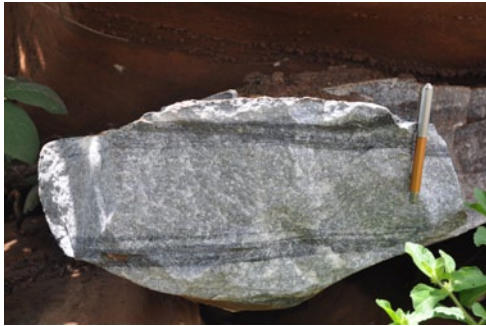
Marble of the Cheta Formation found in the Upper Chalimbana Catchment with a sugary surface and crystalline texture and darker bands
