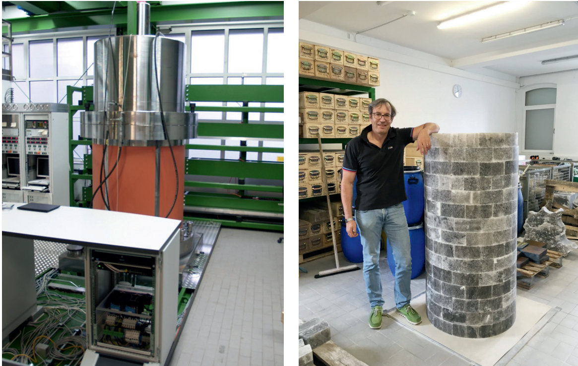
Figure 3.1: Test device for the large-scale pilot plant (left) and stonework made of salt bricks (right)
