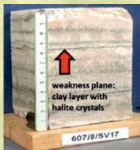
Sample preparation for the direct shear test, already collapsed into two parts before the shear test
